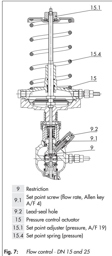
7. Guide the wire through the lead-seal hole (9.2) and lead-seal it to fix the adjusted flow rate.
