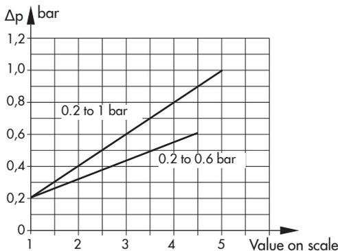
Fig. 11: Differential pressure set point adjusted according to the value on the scale · DN 15 and 25
