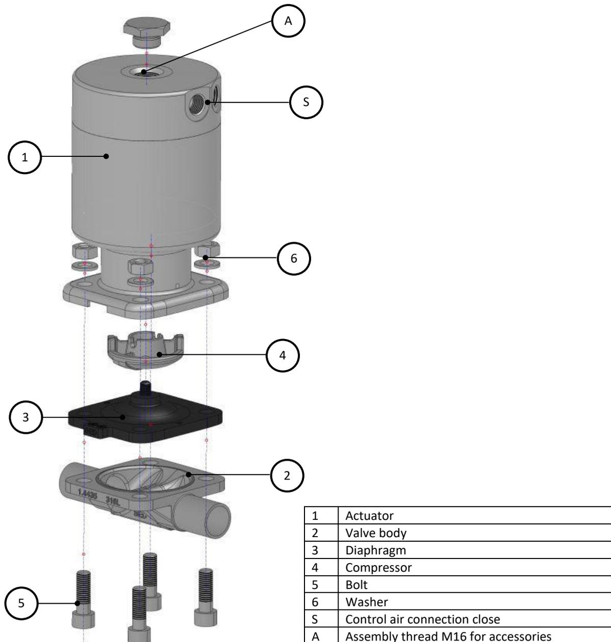
The control air connections are dependent on the control function of the actuator.
