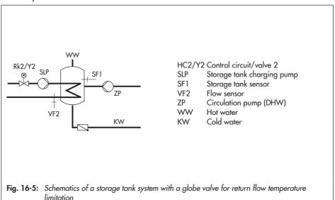
Globe valve and flow sensor VF2 are used exclusively for return flow temperature limitation in the schematics shown above. The pre-control circuit provides at least the same flow temperature as in the standard schematic version which is calculated from 'DHW temperature set
