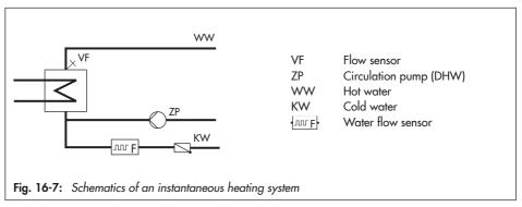
When the rate of hot water being tapped is not being measured: the control of the required 'DHW temperature' at the flow sensor VF is only active during times-of-use of the circulation pump ZP. To measure the rate of hot water being tapped, the setting CO4 -> F04 - 1 allows either a flow switch, a water flow sensor (1400-9246) or a vortex flow sensor to be activated. The vortex flow sensor must be powered by an external source (usually 5 V).
