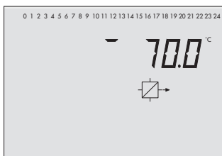
Flow sensor VF1, primary heat exchanger circuit
