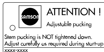
Fig. 4: Label when an adjustable packing is installed
