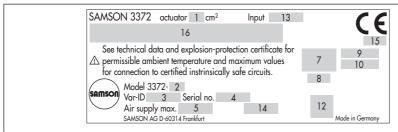
Fig. 2-2: Nameplate of Type 3372 Actuator with integrated i/p converter in explosion-protected version
