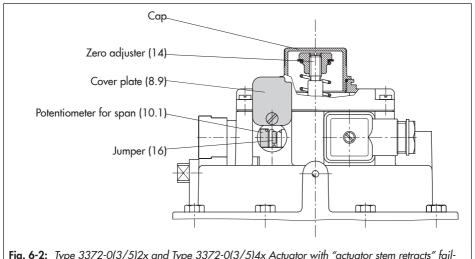
Fig. 6-2: Type 3372-0(3/5)2x and Type 3372-0(3/5)4x Actuator with "actuator stem retracts" failsafe action
