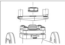
Fig. 3-1: Mounting using a central nut (form B attachment)
