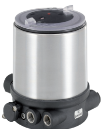
024.16.7 Electropneumatic positioner 4-20 mA for pneumatically actuated valves with single or double acting actuator Operating voltage 24 V Central mounted and also for retrofitting microprocessor controlled electronics for signal processing, actual/setpoint optional as process controller with PID qualities.
