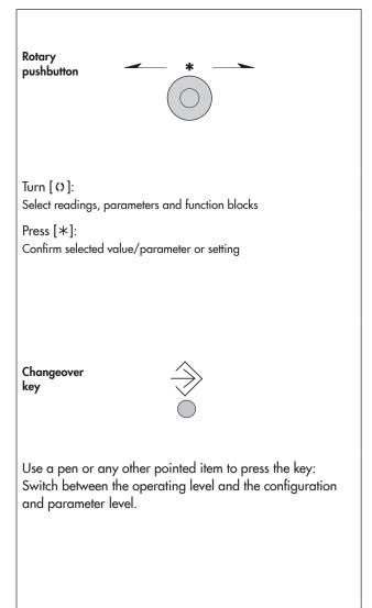
Fig. 2: Rotary pushbutton and changeover key
