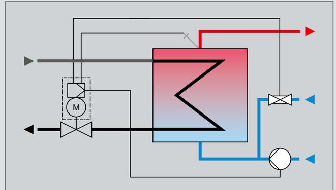
Standard application for domestic hot water heating in instantaneous heating systems with tapping detection and pump control
